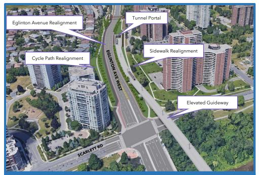
To make room for the tunnel boring machine extraction shaft and the tunnel portal, a section of Eglinton Avenue West will be realigned to the south between the pedestrian bridge and Scarlett Rd. Realignment work begins in Spring 2022.
